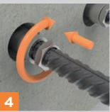
Screw the coupler by hand onto the 1st phase rebar.
