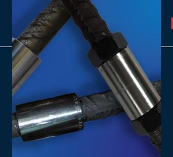
However, BS 8110 Clause 3.12.8.16.2 Bars in tension states "The only acceptable form of full-strength butt joint for a bar in tension comprises a mechanical coupler" satisfying specified slip and tensile strength criteria.
